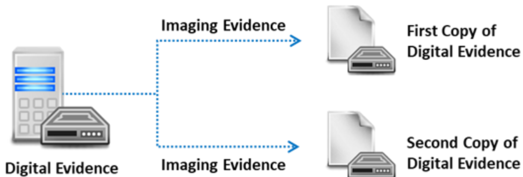
Figure 4.7: Data acquisition using imaging tools
